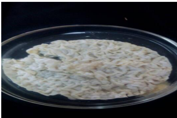
Figure 37 Image of cellulose biofilm by G. xylinus under static condition (see online version for colours)
