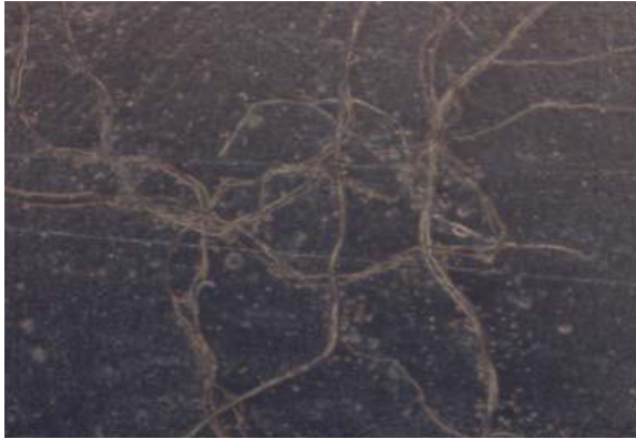
Figure 7 Phase contrast images of fibrous structure of biocellulose (see online version for colours)
