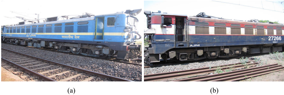
Figure 1 (a) CLW make WAG7 (b) BHEL make WAG7 (see online version for colours)
