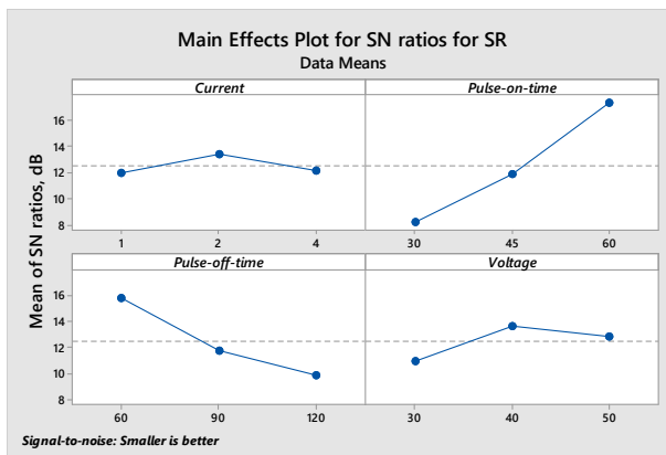
Figure 5 S/N ratios plot for effects of machining parameters on SR (see online version for colours)
