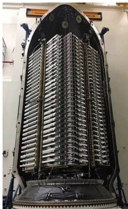
Figure 7 SpaceX 60 stars loading structure (see online version for colours)
