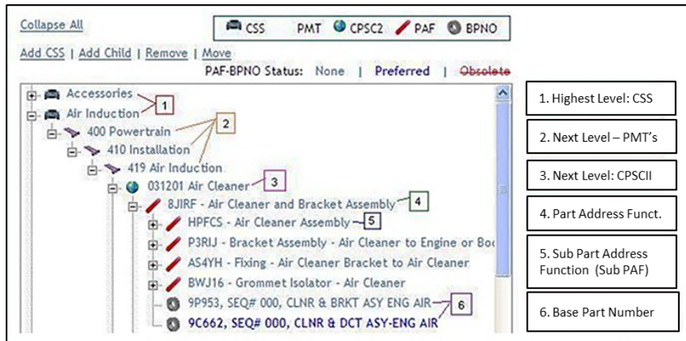
Figure 3 Vehicle architecture structure – six-level hierarchy (see online version for colours)
