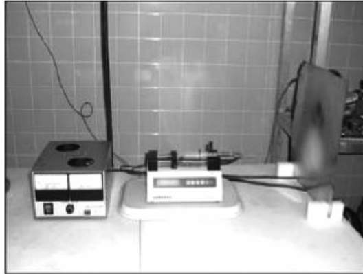
Figure 4 Photographic image of the electrospinning setup
