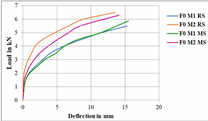
**Figure 4** Load vs. deflection: 0.2% foaming agent (see online version for colours)
