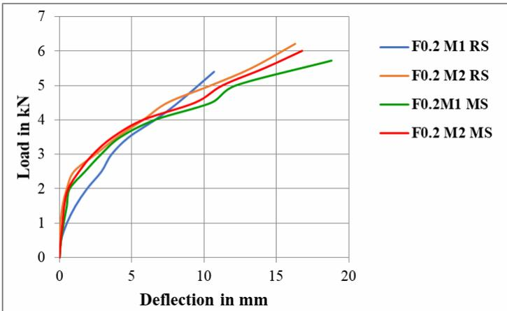
**Figure 5** Load vs. deflection: 0.4% foaming agent (see online version for colours)
