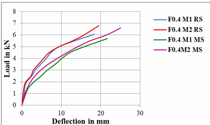
**Figure 6** Load vs. deflection: 0.6% foaming agent (see online version for colours)
