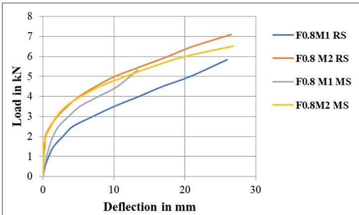
**Figure 8** Load vs. deflection: 1% foaming agent (see online version for colours)
