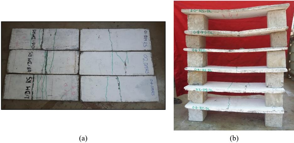
**Figure 13** (a) Crack pattern: M<sub>1</sub>MS (b) Deflected shapes: M<sub>1</sub>MS (see online version for colours)
