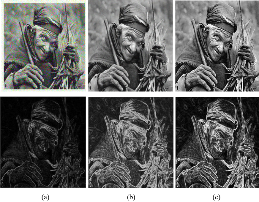
Figure 11 Edge detection on a pre-processed image from internet, (a) noisy image (b) smoothed image (c) enhanced image (see online version for colours)
