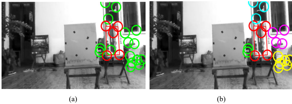
Figure 10 Isolation technique for the detected feature points, (a) convex hull is formed from the obstacle region feature points (b) the free region feature point inside the convex hull is removed (see online version for colours)
