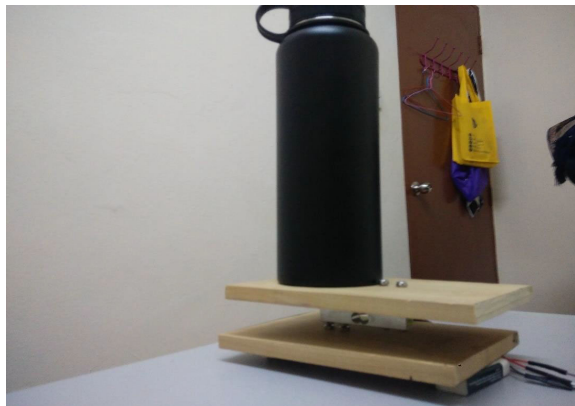
Figure 5 Load cell sensor with wooden base with flask as the cylinder (see online version for colours)
