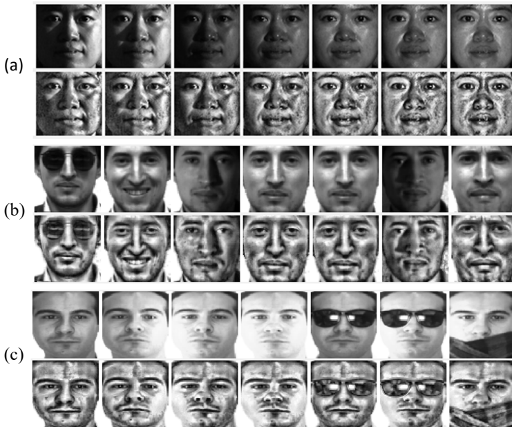
Figure 2 CLAHE enhancement results on, (a) CMU PIE (b) Yale database (c) AR database (see online version for colours)
