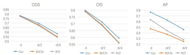
Figure 8 On the BSDS500, the MHANet, RCF and BDCN have different maximum tolerance distances d for the increasing and decreasing trends in the evaluation indexes (ODS, OIS, and AP) (see online version for colours)
