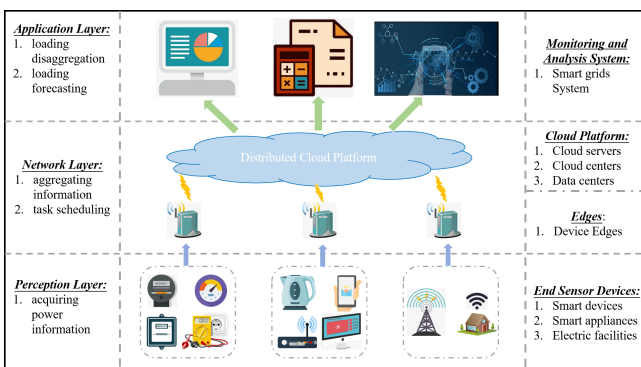
Figure 1 Structure diagram of IoT-enabled distributed smart grids (see online version for colours)
