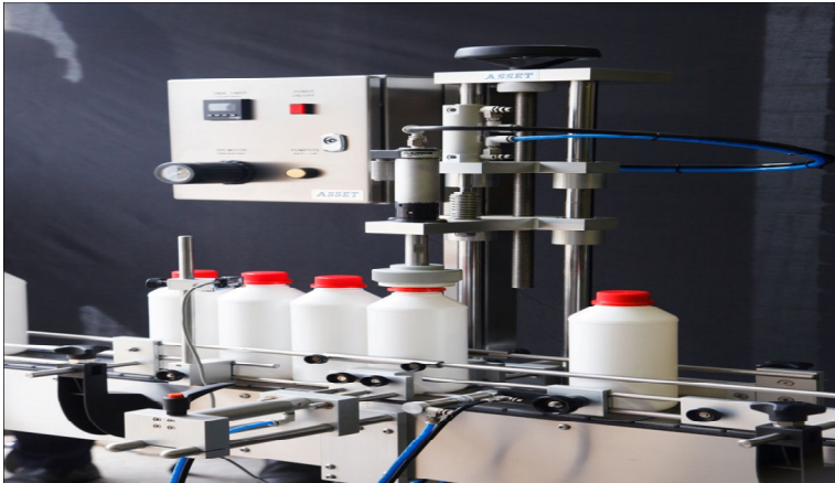
Figure 1 A device that fixes a bottle cap (see online version for colours)
