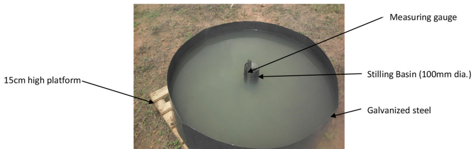
Figure 1 An installed evaporation pan for the measurement of daily evaporation (mm/day) (see online version for colours)
