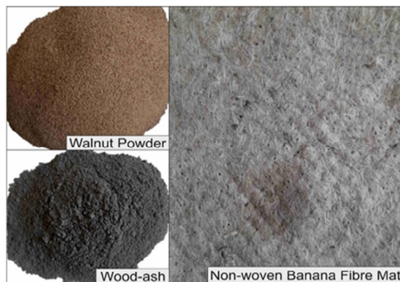
Figure 1 Pictorial view of non-woven (banana) fibre, walnut powder, and wood ash (see online version for colours)
