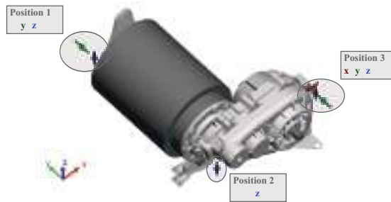
Figure 9 Position sensor locations at the Twizy ERAD (see online version for colours)
