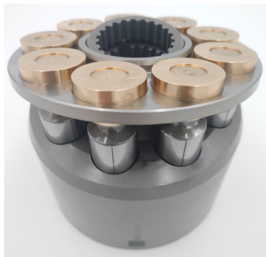
Figure 6 Rotating group of the faulty pump containing nine defective pistons (see online version for colours)
