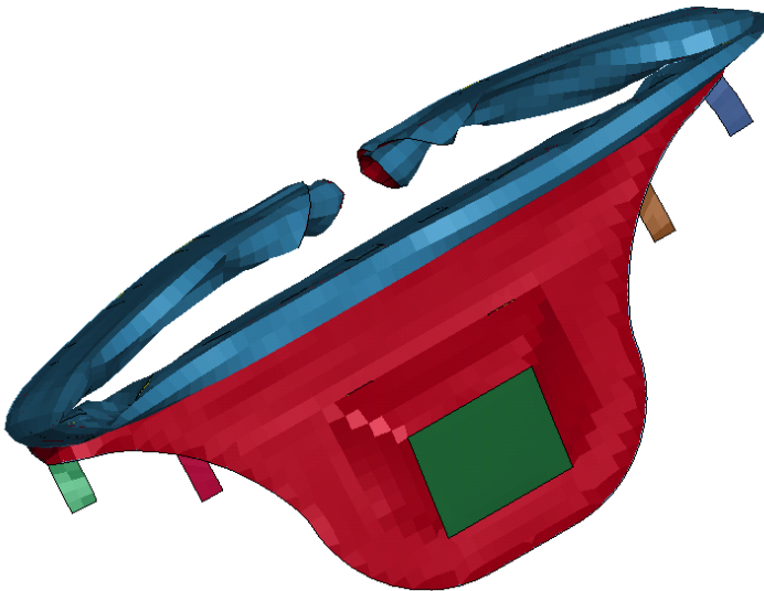
Figure 10 Rolled-Folded pedestrian protection airbag
