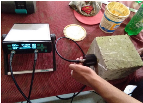
Figure 3 UPV test being conducted on a concrete cube (see online version for colours)
