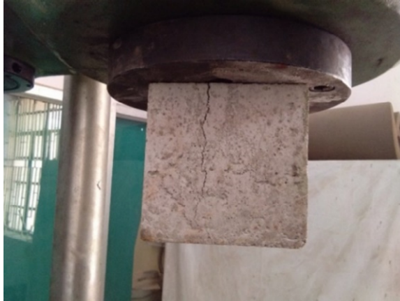
Figure 10 Crack propagation during pull out test (see online version for colours)
