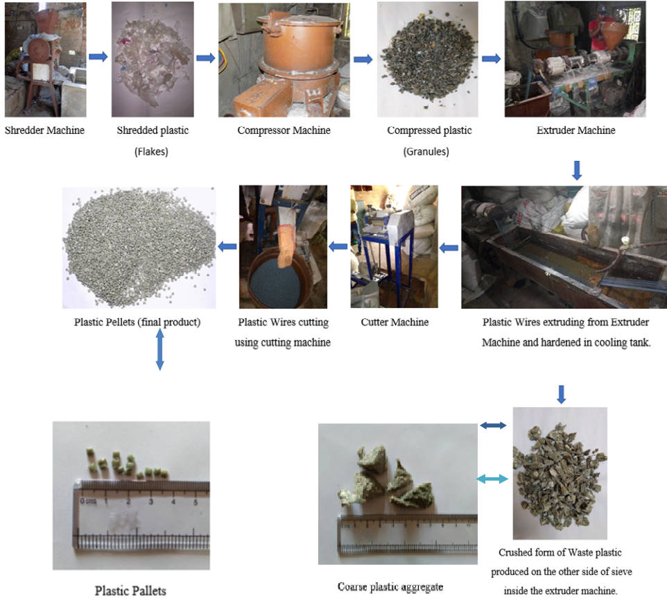
Figure 1 The process of recycling of plastic waste (see online version for colours)
