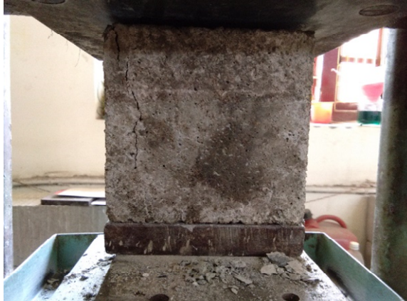
Figure 4 Compressive strength test of a concrete cube containing plastic aggregate (see online version for colours)
