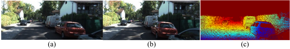
Figure 1 Examples of KITTI stereo dataset. (a) the left image of the scene. (b) the right image of the scene and (c) the disparity image of the scene (see online version for colours)
