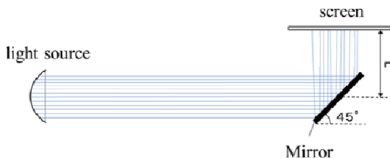
Figure 13 Arrangement of light in ray tracing simulation (see online version for colours)
