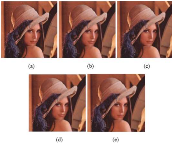
Figure 6 Lena: (a) input image with \sigma = 5 , and p = 0.05 , (b) bilateral filter applied image, (c) trilateral filter applied image, (d) trilateral filter with belief propagation applied image and (e) proposed method image (see online version for colours)
