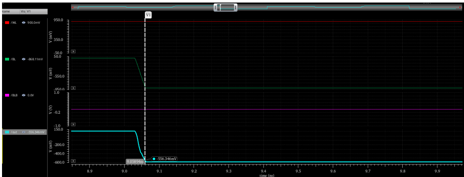
Figure 14 Write delay of 6T SRAM cell (see online version for colours)
