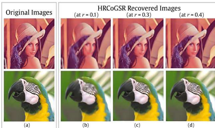
Figure 17 Performance comparison of the colour image recovery with proposed HRCoGSR method for lower sampling ratio (at r = 0.1 ) and higher sampling ratio (at r = 0.3 and 0.4) (see online version for colours)
