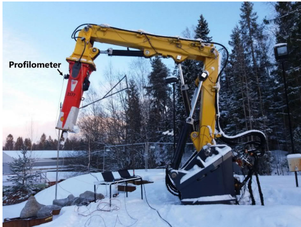
Figure 5 Profilometer installed on a hydraulic breaker boom (see online version for colours)
