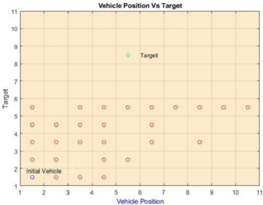
Figure 5 Path searching using A* algorithm
