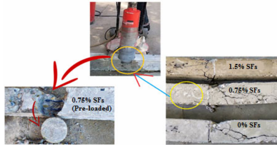
Figure 4 Typical core cross-sectional view of pre-loaded specimens with (a) 0% SFs, (b) 0.75% SFs, (c) 1.5% SFs (see online version for colours)
