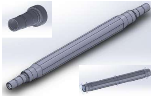
Figure 2 3D model of the failed rear axle beam (see online version for colours)
