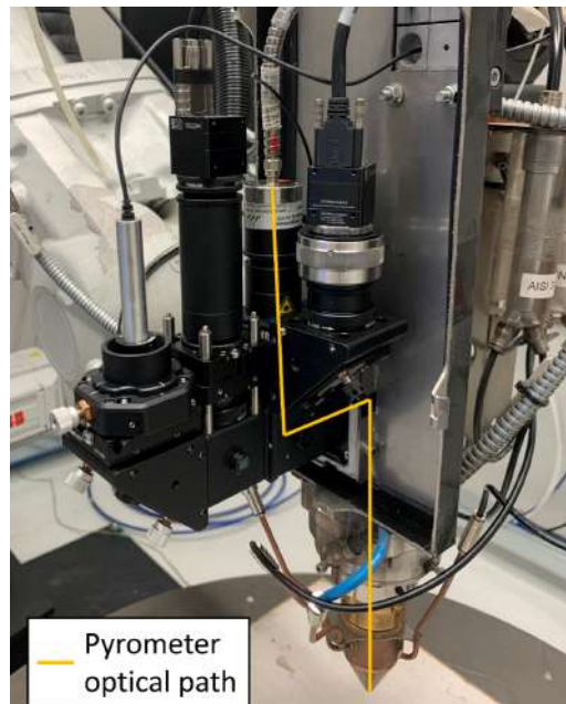
Figure 3 Hardware implementation of the monitoring system on the deposition head. The optical path of the pyrometer is also traced (see online version for colours)
