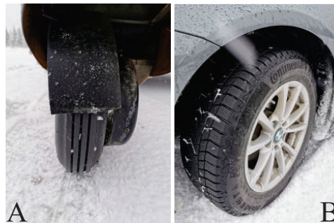
Figure 1 Trelleborg T520 tyre (A) and a standard studless winter tyre (B) (see online version for colours)
