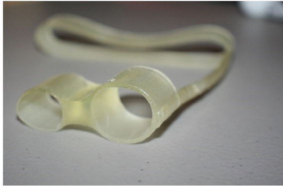
Figure 2 Composite foot support comprised of flexible polymer (3D printed) and inserted support metal. the support is designed to provide maximum correction with the least amount of interference with everyday life (see online version for colours)
