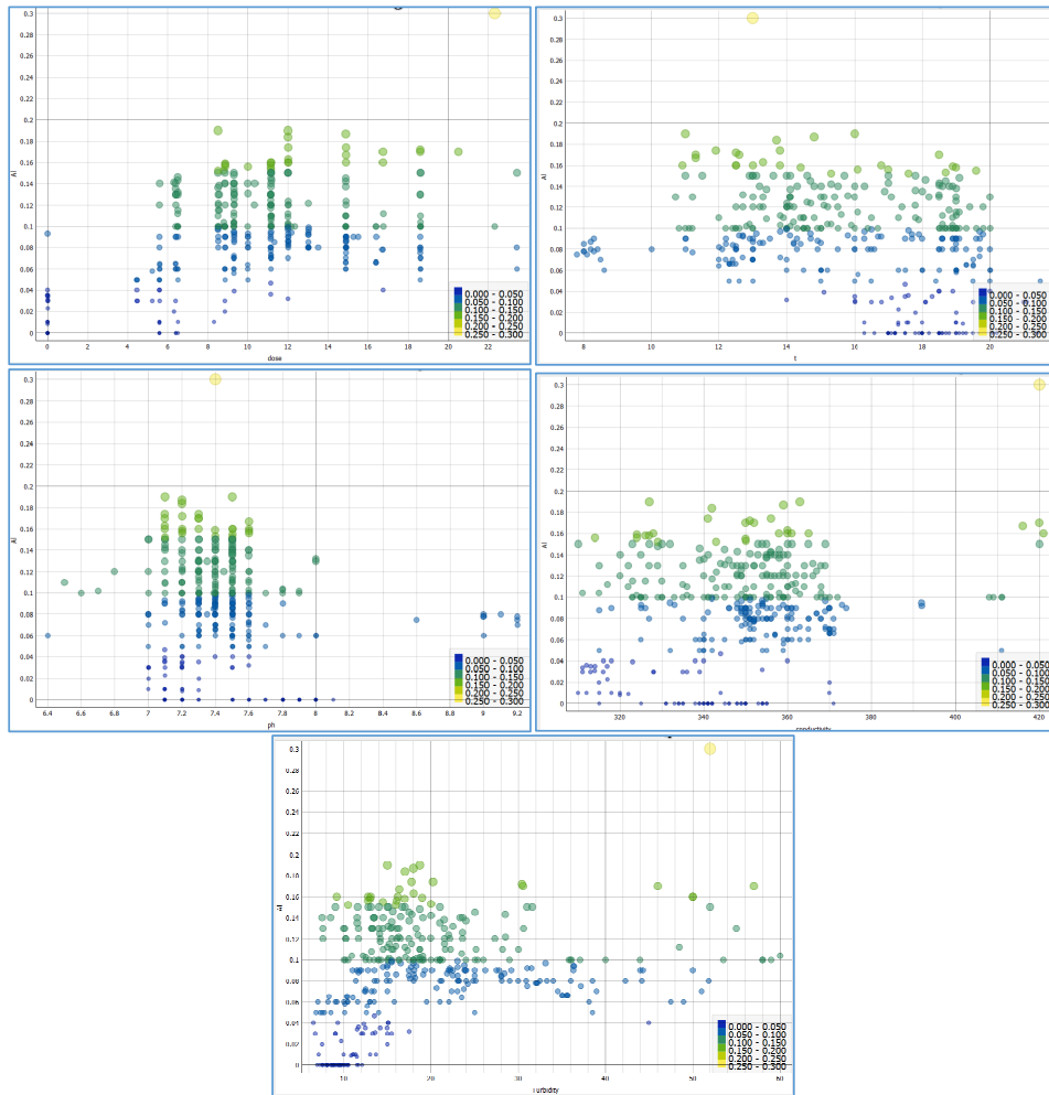
Figure 3 Relation between different parameters and the residual aluminium (see online version for colours)
