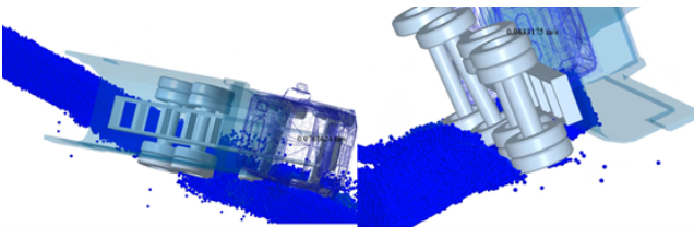
Figure 21 SIM.019 – Leira.001 – impact condition: speed 30 km/h – impact angle 15° – GVW load condition (see online version for colours)
