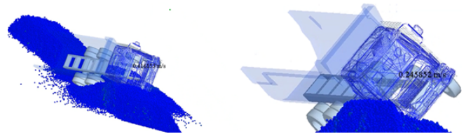
Figure 18 SIM.010 – Naves.005 – impact condition: speed 60 km/h – collision angle: 15° – GVW load condition (see online version for colours)
