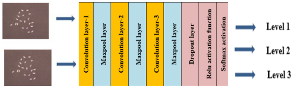
Figure 7 Customised CNN model used for classification of DOM (see online version for colours)
