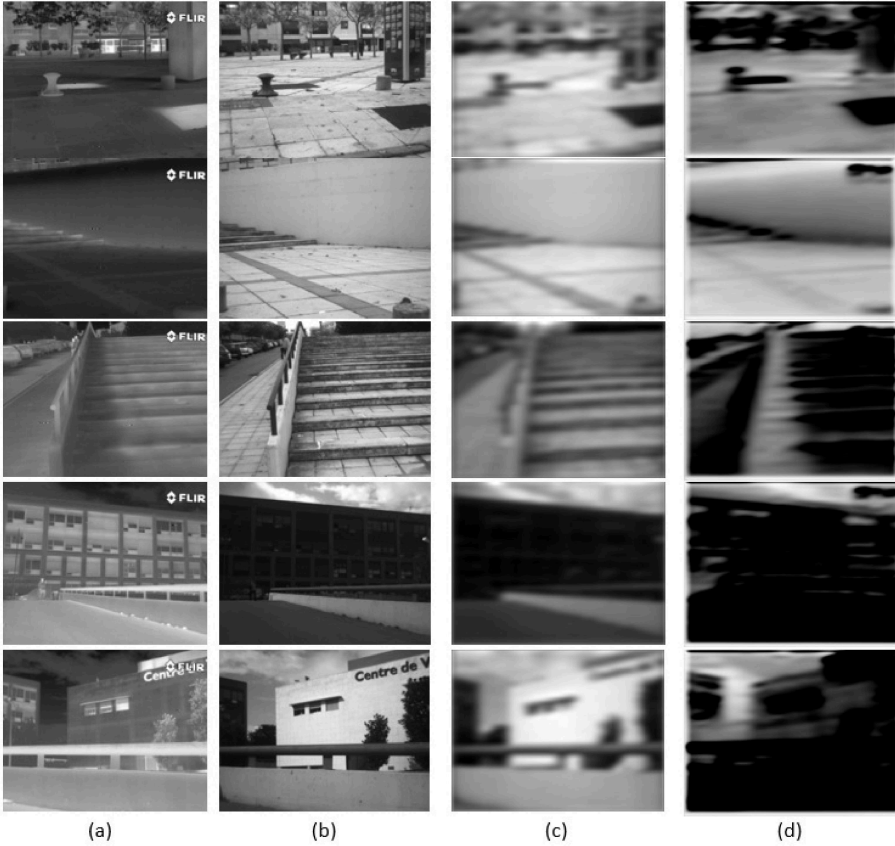
Figure 2 Sample images, (a) original LWIR (b) original visible images (c) unimodal-net VS encoded representative images (d) encoded representative images from multi-modal-net with SSIM loss
