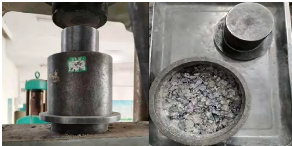
Figure 4 Aggregate crushing value test (see online version for colours)
