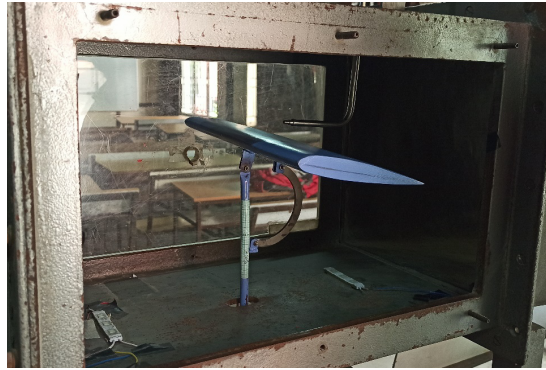
Figure 11 Wing model in the test section (see online version for colours)
