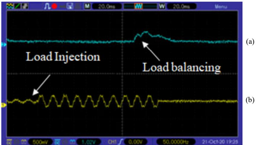
**Figure 16** Load balancing operation of (a) source current and (b) load current in real time (see online version for colours)
