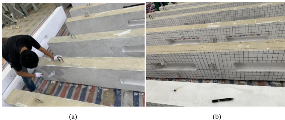
Figure 5 Beam surface treatment, (a) whitening treatment of beam surface (b) drawing grid of beam surface
