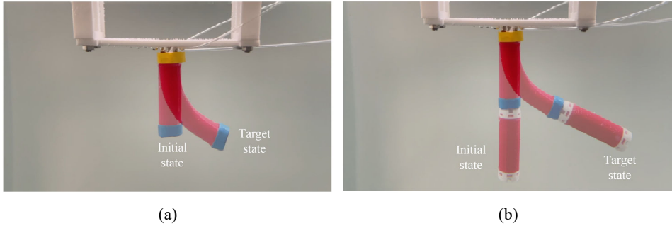
Figure 3 State of modular soft fluidic actuator, (a) single actuator without load, (b) single actuator with load (see online version for colours)
