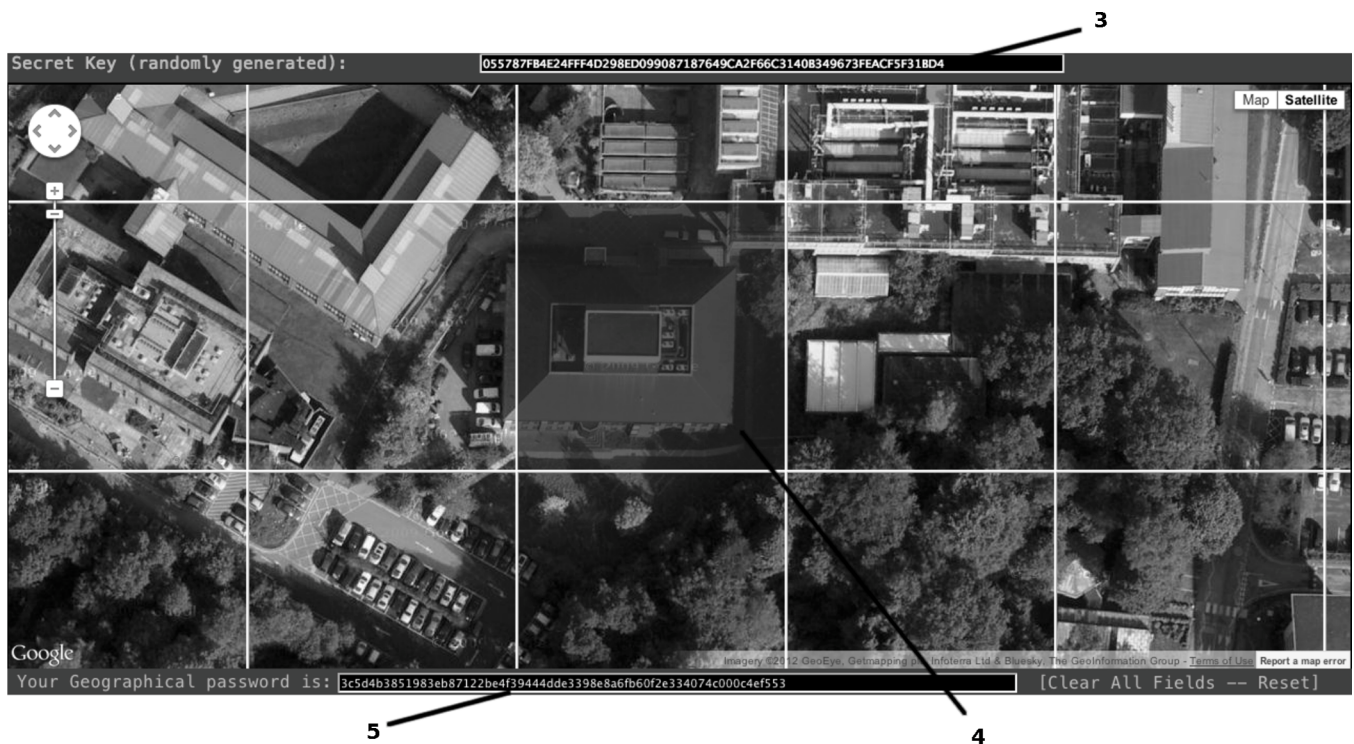
Figure 5 User selecting a geographical location, by selecting a rectangle containing Royal Holloway, Univ. of London library building in UK (4) as her geographical password and transforming it into a keyed hash value (5), where the secret key is 128-bit of length and is randomly generated (3)
