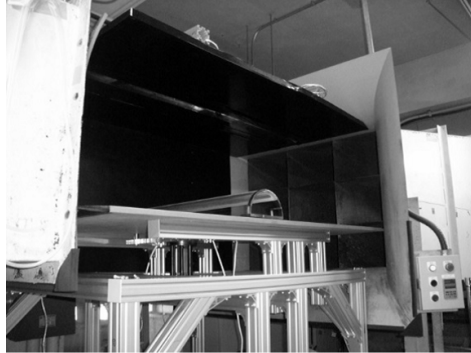
Figure 6 Test section of the wind tunnel
