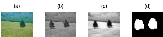
Figure 5 Copy-move forgery detection: (a) original image; (b) grey-scale forgery image of (a); (c) Fuzzy Transform image and (d) forgery detection (see online version for colours)
