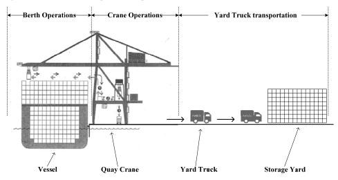
Figure 1 Process of main operations in port area
