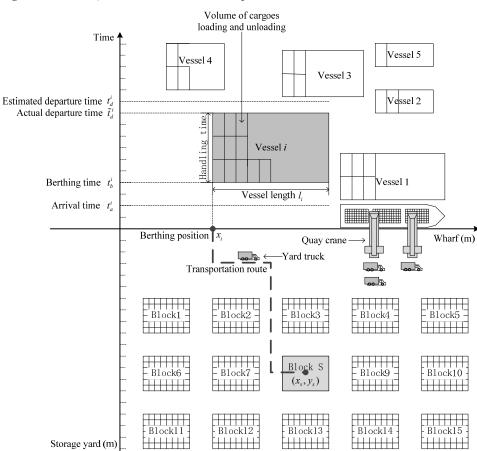
Figure 2 The B-QC-YTAP in two-dimensional plane
