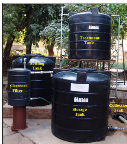
Figure 3 Field setup for chemical treatment of effluent water (see online version for colours)
