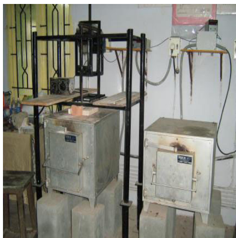
Figure 1 Stir casting setup with mechanical stirrer (see online version for colours)
