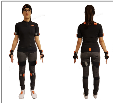
Figure 5 Placement of motion trackers on human body (see online version for colours)
