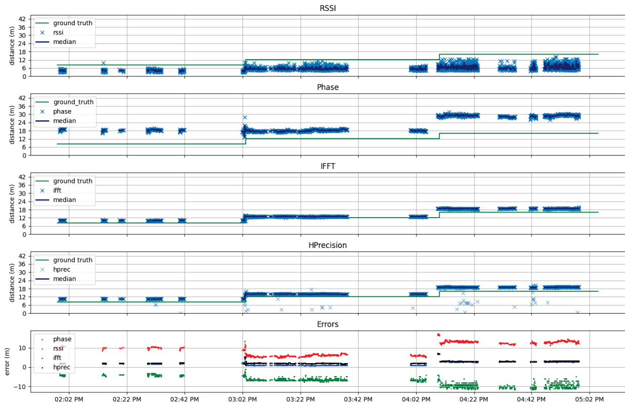
Figure 8 Line of sight distance estimation experiment. Ground truth distances (green), distance estimations provided by each of the methods (light blue), and estimated distances after filtering (dark blue) are shown. The last graph shows the differences between estimated and ground truth distances (see online version for colours)
