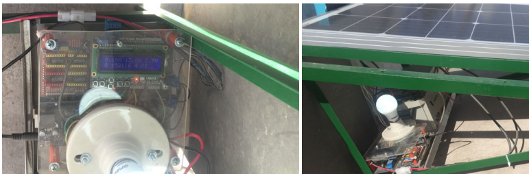
Figure 1 Power (W), amperage (A) and voltage (V) evaluation module (see online version for colours)
